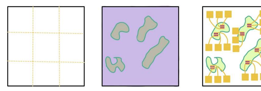
1. Original substrate 3. ALD Deposition 5. Electrodes
