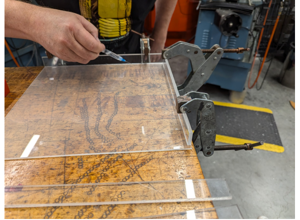
Figure 8: Created an acrylic 12" x 12" tank
